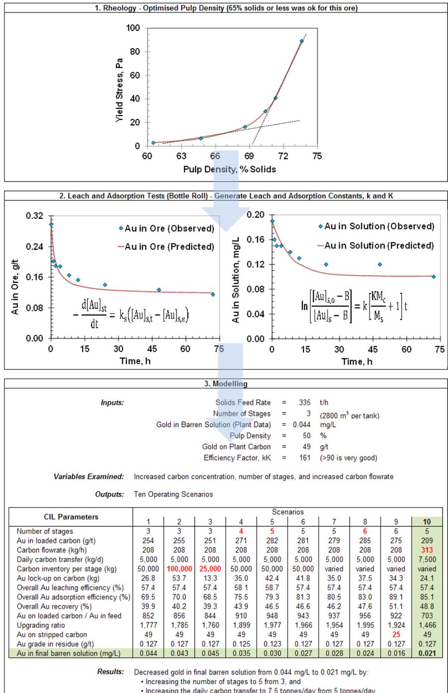
Example: CIL plant in Northern Ontario, Canada that treats low grade gold ore flotation tailing.
